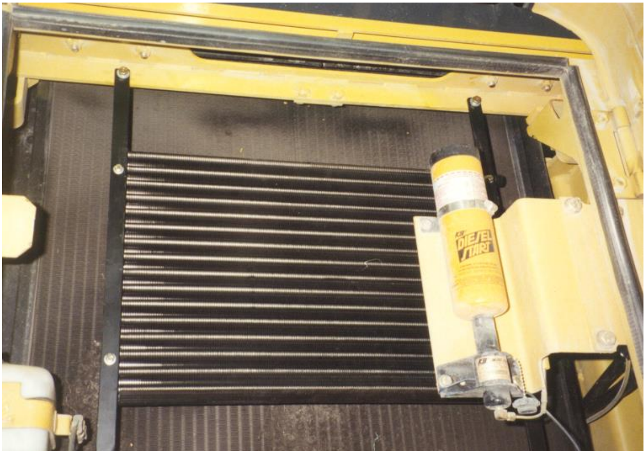
Condenser and brackets mounted in location.
